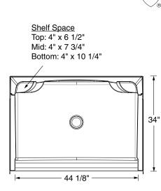
FEATURES Ibs Dimensional Tolerance ± 3/6". Dimensions needed for site preparation should be measured from the unit. Aquatic assumes no responsibility for preparatory work.
