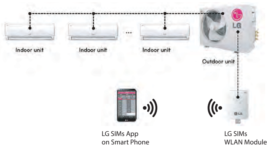
Figure 76: SIMS WLAN Module to Typical DFS System
