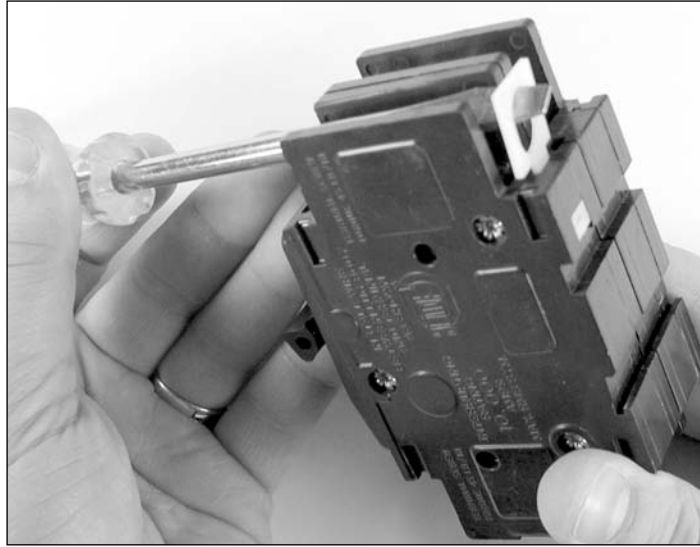
FIGURE 5 ROTATING CIRCUIT BREAKER
